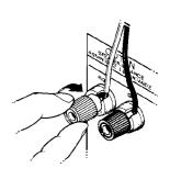
**CAUTION:** Two speaker systems can be connected to this unit. The minimum speaker impedance should be  $4\Omega$  when only one speaker system is connected. When two speaker systems are connected, care should be taken that net impedance does not become less than  $4\Omega$ .
